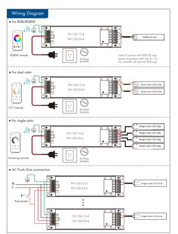
Note: Long press match key 5s, then short press match key 3 times, the light on/off time will be set to 3s, the indicator light blink 3 times. Long press match key 10s, restore factory default parameter, the light on/off time also restore to 0.5s.
